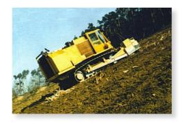
The KMMCS can easily manage gradients up to 40° forwards or backwards.
