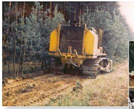
Vegetation of up to 30 cm in diameter and more is no obstacle and gets embedded into the soil.
